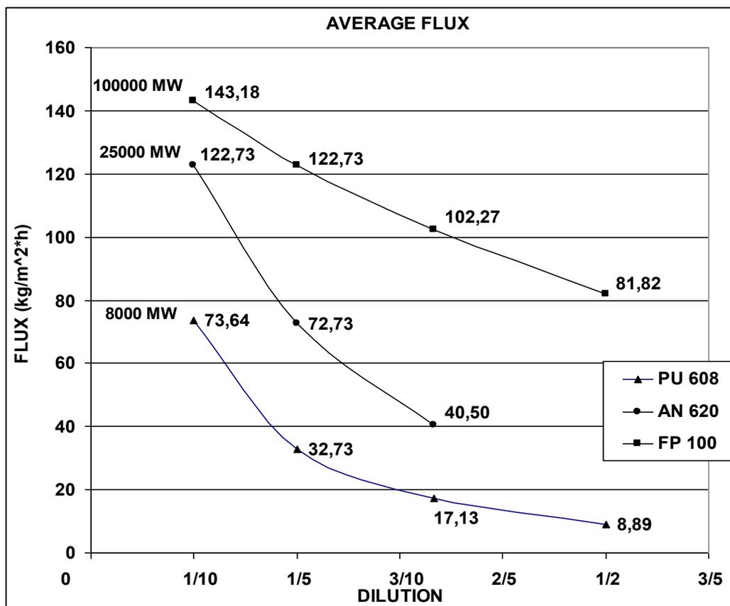
**Figure 1.:** Average Diafiltration flux at optimum conditions (temperature  $60^\circ\text{C}$  And trans-membrane pressure 4 bar) vs. OMWW dilution.
