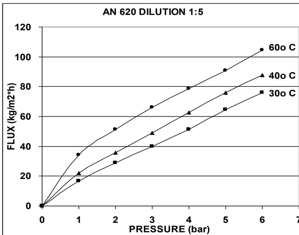
**Figure 2.:** OMWW Diafiltration flux vs operating temperature.
