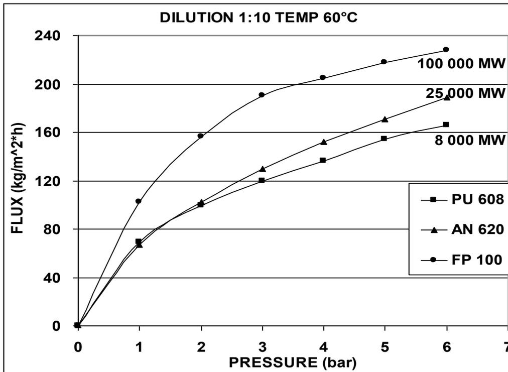
**Figure 3.:** OMWW Diafiltration flux at 1/10 dilution and 60°C vs applied transmembrane pressure for different membranes.
